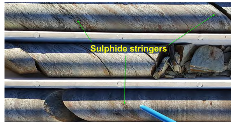
Figure 9: Diamond drill core with uncut disseminated (stringer?) base metal mineralization, Conquistador Prospect
